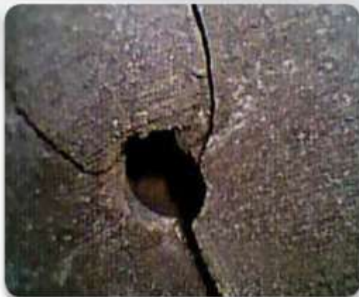
Using the optional Close-Focus Tip, fine cracks are detected inside a combustion chamber.
